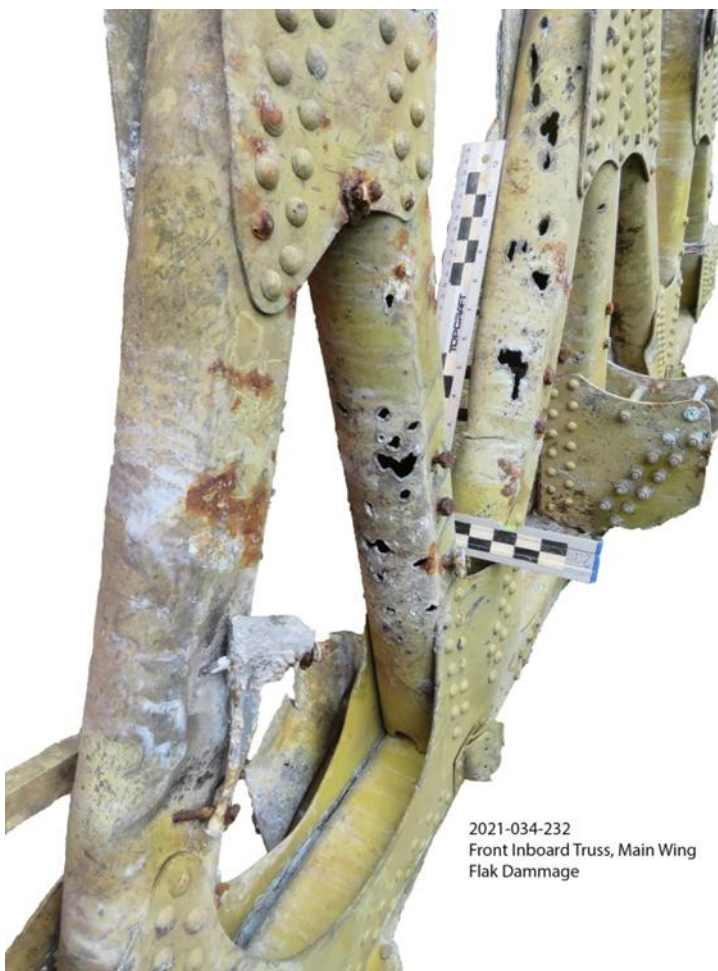
Plt-13, Shrapnel damage, wing truss support
